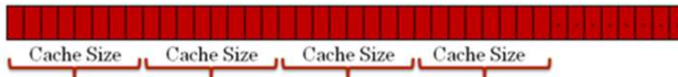
Figure 3: Cache-efficient parallel sort first stage. Each cache sized block is sorted followed by parallel merging
