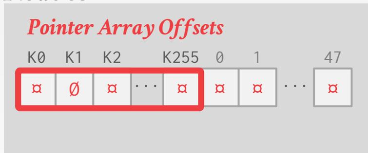
Instead of storing 1-byte digits, maintain an array of 1-byte offsets to a child pointer array that is indexed on the digit bits.
