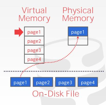
One can use memory mapping (mmap) to store the contents of a file into a process' address space.
